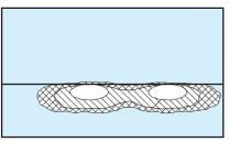
5. Locate the vertical adjuster on the headlamp, then turn the adjuster either clockwise (to adjust up) or counterclockwise (to adjust down) aligning the upper edge of the light pattern to the horizontal line.
